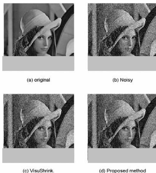
Fig. 3. a) Original image of Lena, b) Image corrupted by a gaussian noise with  $\sigma_n = 38.25$ , c) VisuShrink method, d) proposed method
