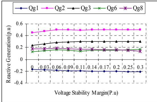
Fig. 8. Reactive power outputs of the generators (Case 2)
