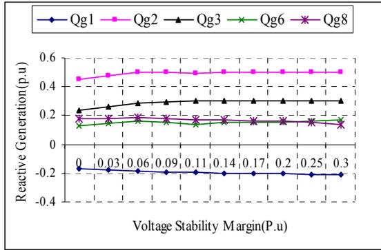
Fig. 17. Reactive power outputs of the generators (Case5)
