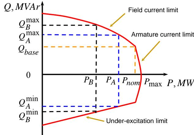
Fig.1. Typical capability curve of a generator [12]
