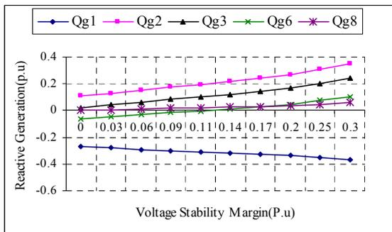
Fig. 14. Reactive power outputs of the generators (Case 4)
