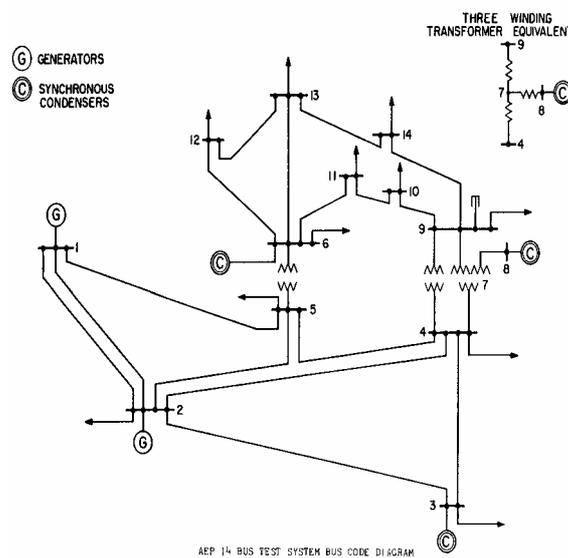
Fig. 4. IEEE 14 bus test system
