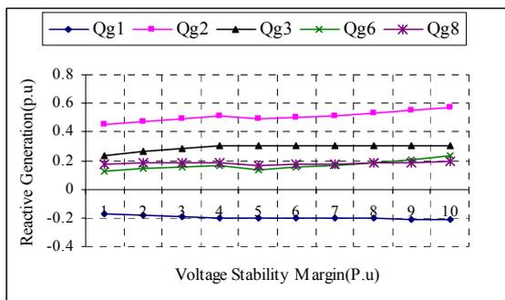
Fig. 11. Reactive power outputs of the generators (Case 3)
