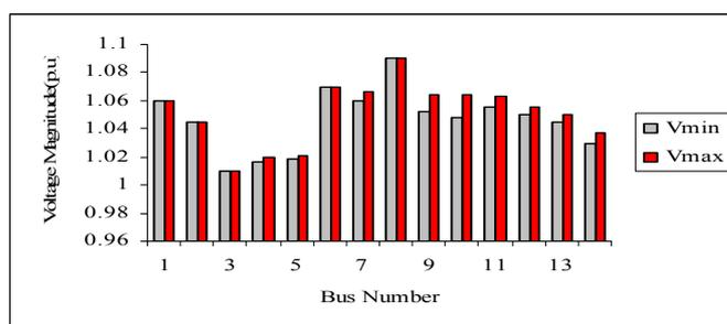
Fig. 7. Voltages variation respect to increasing vsm (Case 1)
