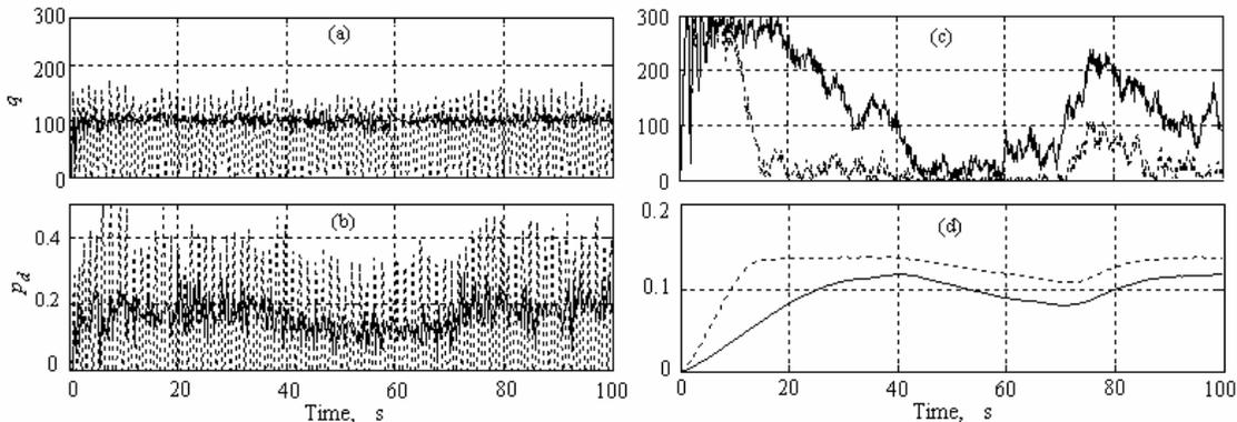
Fig. 7. Queue length and marking probability evolution for Exp. 2, (a) and (b): ARM-PFC (line), RED (dot); (c) and (d): PI (line), REM (dot)
