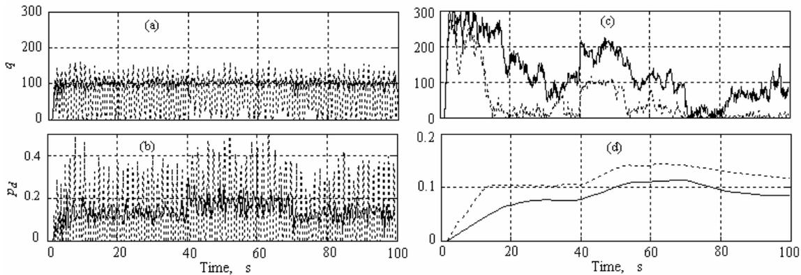
Fig. 10: Queue length and marking probability evolution for Exp. 5, a) and b): ARM-PFC (line), RED (dot); c) and d): PI (line), REM (dot)
