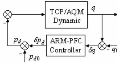
Fig. 3. Block diagram of ARM-PFC as an AQM method
