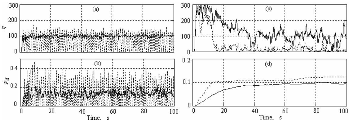
Fig. 14. Queue length and marking probability evolution for Exp. 8, a) and b): ARM-PFC (line), RED (dot); c) and(d): PI (line), REM (dot)
