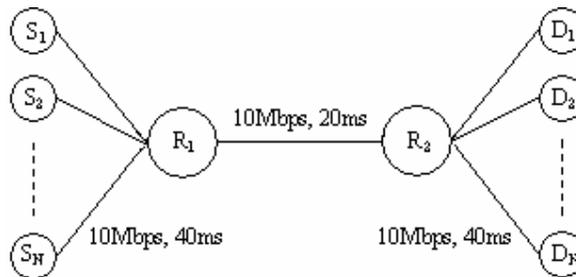
Fig. 4. Dumbbell network topology for  $ns-2$  simulations
