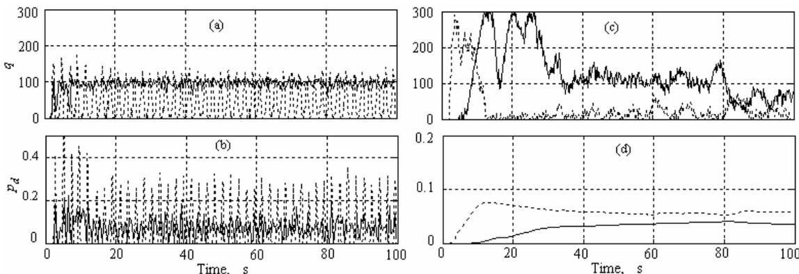
Fig. 12. Queue length and marking probability evolution Exp. 6 for much larger RTT, a) and (b):ARM-PFC (line), RED (dot); (c) and(d): PI (line), REM (dot)
