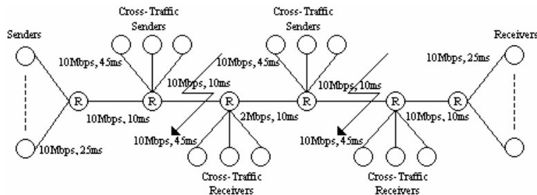
Fig. 5. Network topology with multiple bottlenecks
