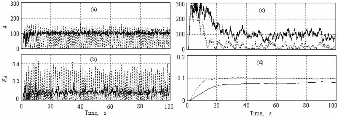
Fig. 6. Queue length and marking probability evolution for Exp. 1, (a) and (b): ARM-PFC (line), RED (dot); (c) and (d): PI (line), REM (dot)
