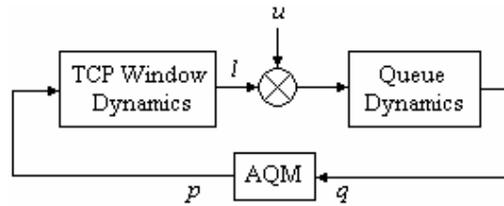
Fig. 2. Block diagram of TCP/AQM network interactions including responsive and unresponsive flows
