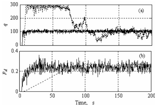
Fig. 9: a) Queue length evolution, b) Marking probability for Exp. 4: ARM-PFC (line), PI (dot)
