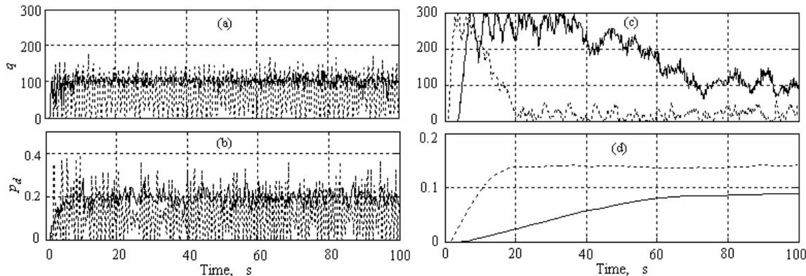
Fig. 11. Queue length and marking probability evolution Exp. 6 for much smaller RTT, a) and b):ARM-PFC (line), RED (dot); (c) and(d): PI (line), REM (dot)
