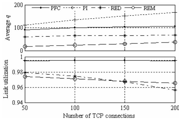
Fig. 8. Average queue and link utilization w.r.t. number of TCP flows (Exp. 3)
