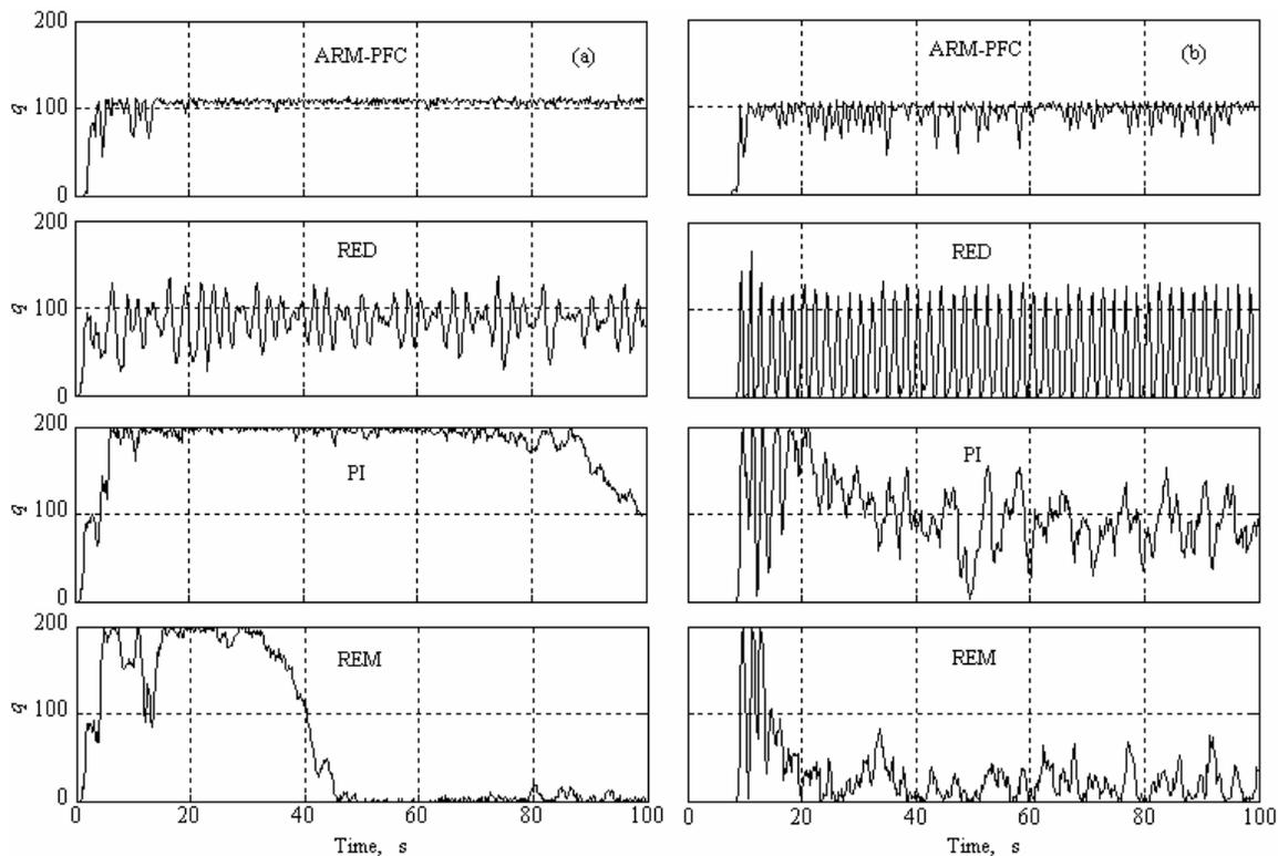
Fig. 15. Queue length evolution for (a) Queue 2 and (b) Queue 4 in the multiple bottleneck scenario
