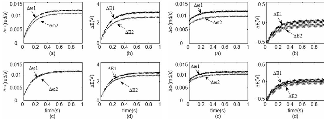
Fig. 17. Frequency and amplitude deviation: a) and b) without the droop controller, c) and d), with the droop controller in supplying a linear load (Left) and a non-linear load (Right) for two UPS inverters 1&2
