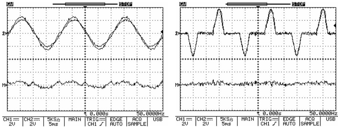
Fig. 19. Experimental results showing the two UPS inverter output currents ( $I_p$ ), and their difference with the droop controller - linear load (Left) and non-linear load (Right) (Ch.1,Ch.2: Current waveforms, X axis: 5ms/div, Y axis: 7A/div Ch.M (MATH=Ch.1-Ch.2): Current waveforms difference, X axis: 5ms/div, Y axis: 7A/div)
