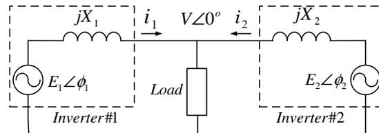
Fig. 2. Equivalent circuit of operation of two inverters
