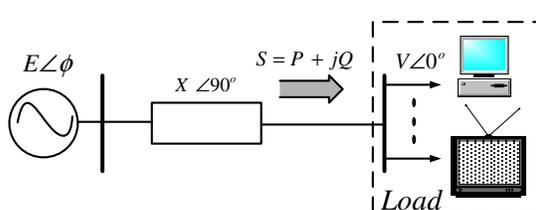
Fig. 1. Equivalent circuit of an inverter connected to a load bus
