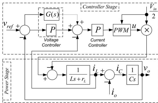
Fig. 5. Block diagram scheme of the single phase inverter output-voltage controller with power circuit stage
