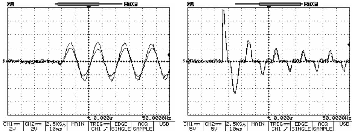
Fig. 22. Experimental result showing the two UPS inverter output currents connected to each other and then sudden connection to a linear load (Left) and a non-linear load (Right) (Ch-1,Ch-2: Current waveforms, X axis: 5ms/div, Y axis: 7A/div(Left) Y axis: 17.5A/div(Right))
