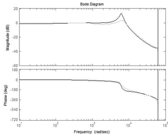
Fig. 6. Bode diagrams of the closed-loop transfer function of the system: with the conventional PID (light trace) and with the PR controller (dark trace)
