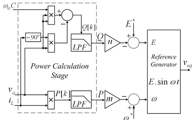
Fig. 8. Improved block diagram of the droop controller
