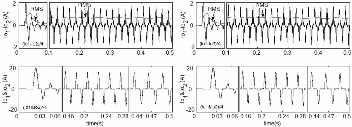
Fig. 14. Transient output current waveforms -with output current sensor (Left) -without output current sensor (Right): (0-20ms) no load and without droop controller, (20ms-180ms) with load and without droop controller, and (180ms-500ms) with load and droop controller; non-linear load
