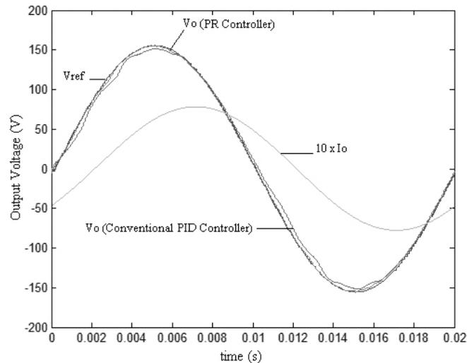
Fig. 7. Comparison of output voltage waveforms using a conventional PID and the PR controller
