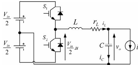
Fig. 4. Power circuit of the single-phase UPS inverter
