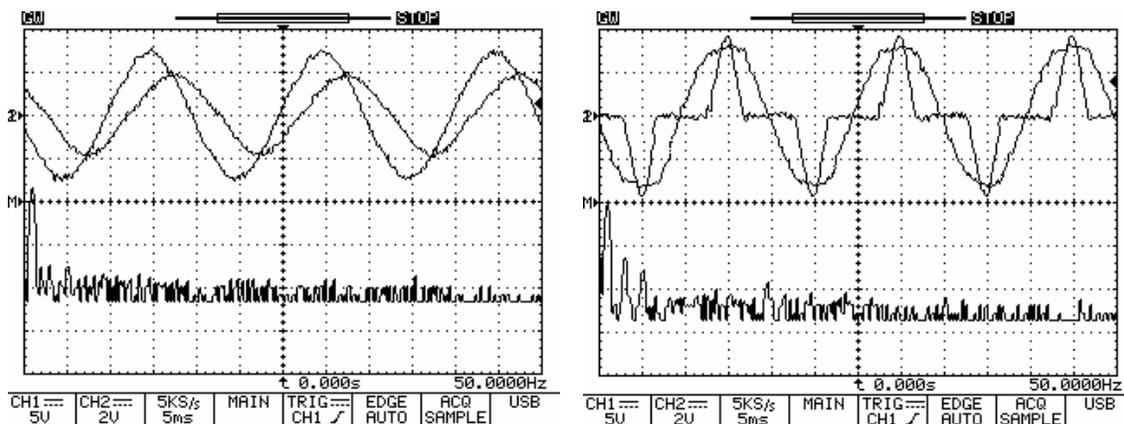
Fig. 21. Experimental result showing the load voltage and its frequency spectrum and load current -linear load (Left) and non-linear load (Right) (Ch.1: Voltage waveforms, Y axis: 100V/div, Ch.2: Current waveform, Y axis: 7A/div, X axis: 5ms/div Ch.M (MATH=Ch.1-Ch.2): Load voltage frequency spectrum, X axis: 250Hz/div, Y axis: 20dB/div)
