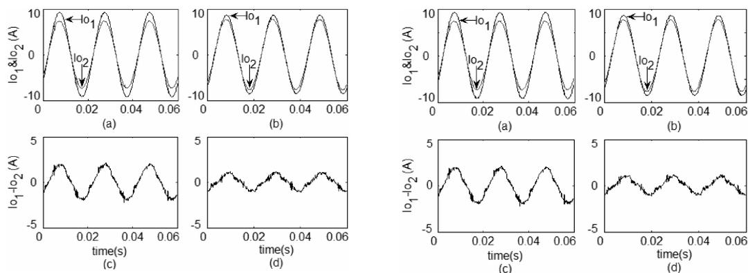
Fig. 10. Steady state output current waveforms and their differences -with output current sensor (Left) -without output current sensor (Right): a) and c) without the droop controller, b) and d) with the droop controller; linear load
