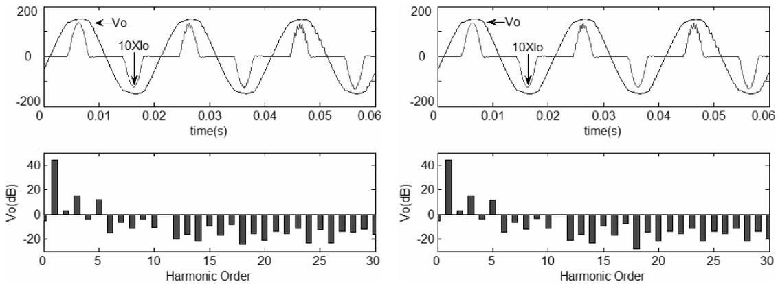
Fig. 15. Output voltage with its spectrum and output current waveforms -with output current sensor (Left) -without output current sensor (Right); non-linear load
