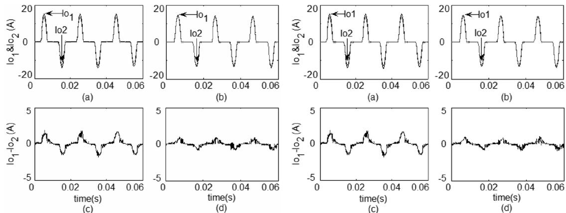
Fig. 13. Steady state output current waveforms and their differences -with output current sensor (Left) -without output current sensor (Right): a) and c) without the droop controller, b) and d) with the droop controller; non-linear load
