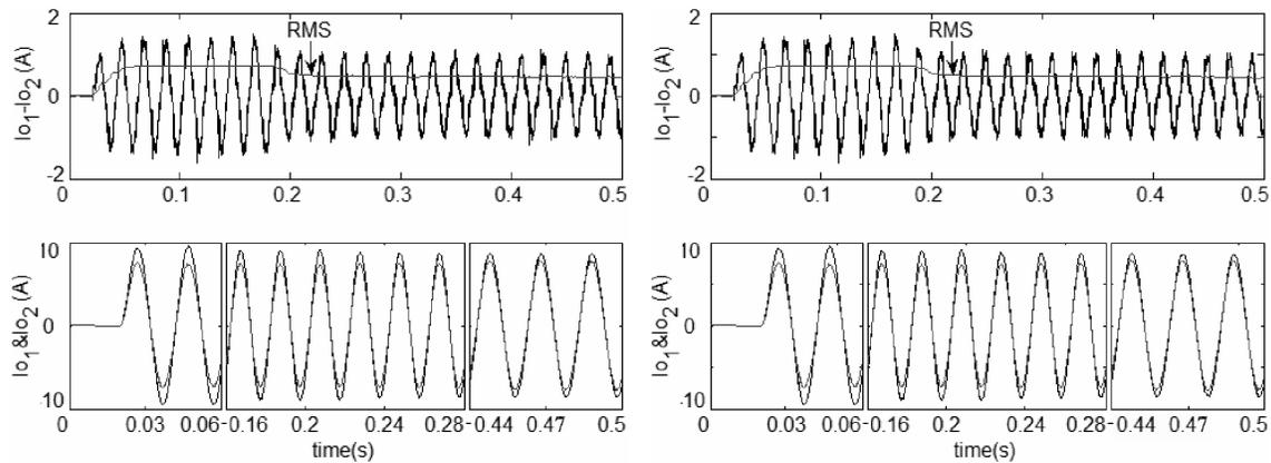
Fig. 11. Transient output current waveforms -with output current sensor (Left) -without output current sensor (Right): (0-20ms) no load and without droop controller, (20ms-180ms) with load and without droop controller, and (180ms-500ms) with load and droop controller; linear load
