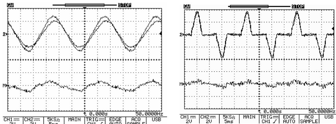
Fig. 18. Experimental results showing the two UPS inverter output currents (Up), and their difference without the droop controller - linear load (Left) and non-linear load (Right) (Ch.1, Ch.2: Current waveforms, X axis: 5ms/div, Y axis: 7A/div Ch.M (MATH=Ch.1-Ch.2): Current waveforms difference, X axis: 5ms/div, Y axis: 7A/div)
