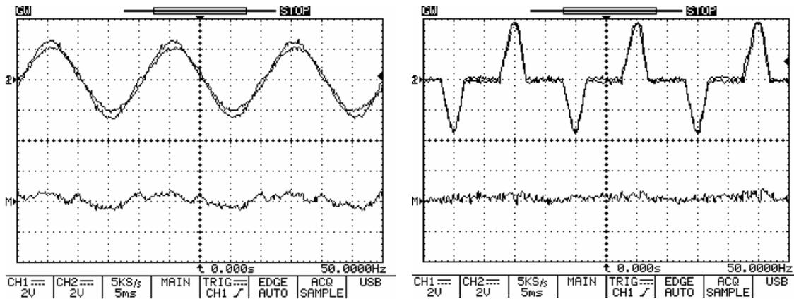
Fig. 20. Experimental results showing the two UPS inverter output currents ( $I_p$ ), and their difference with the droop controller and no output current sensor - linear load (Left) and non-linear load (Right) (Ch.1, Ch.2: Current waveforms, X axis: 5ms/div, Y axis: 7A/div Ch.M (MATH=Ch.1-Ch.2): Current waveforms difference, X axis: 5ms/div, Y axis: 7A/div)
