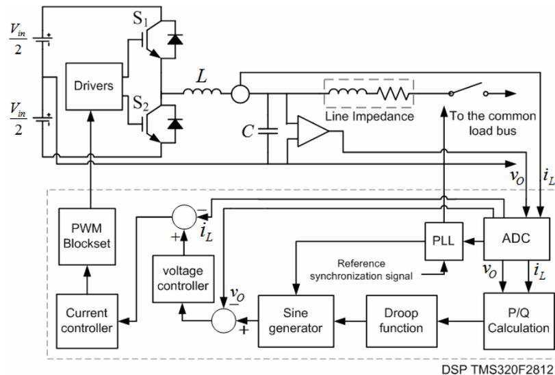
Fig. 9. Block diagram of the power sharing controller
