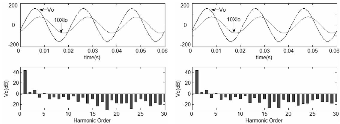
Fig. 12. Output voltage with its spectrum and output current waveforms -with output current sensor (Left) -without output current sensor (Right); linear load
