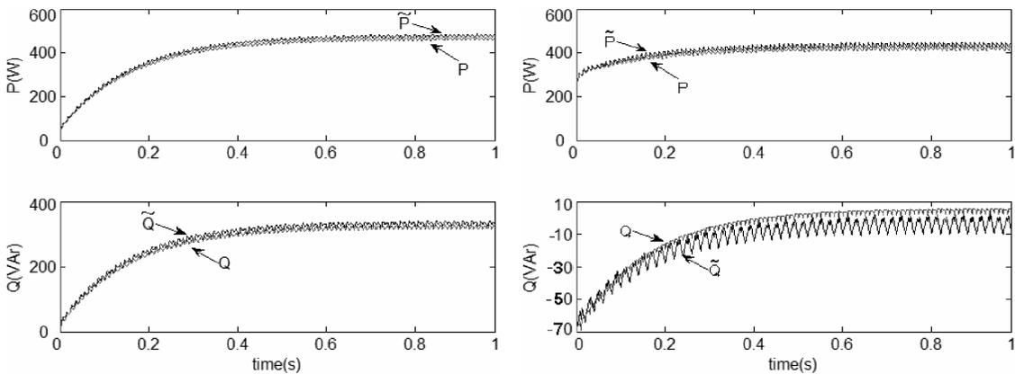
Fig. 16. Waveforms of active and reactive power: without the output current sensor ( $\tilde{P}, \tilde{Q}$ ) and with the output current feedback ( $P, Q$ ) in supplying a linear load (Left) and a non-linear load (Right)
