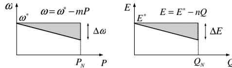
Fig. 3. Static droop characteristic  $\omega - P$  and  $E - Q$
