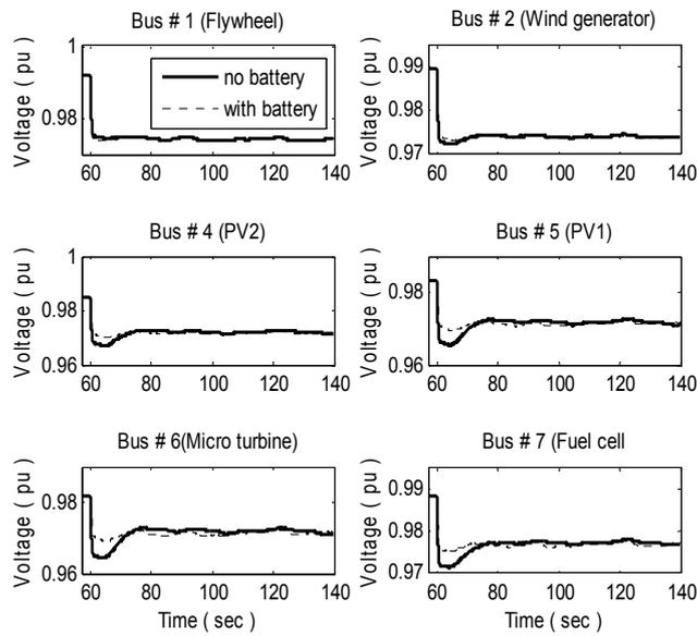
Fig. 9. Voltages at all micro sources buses
