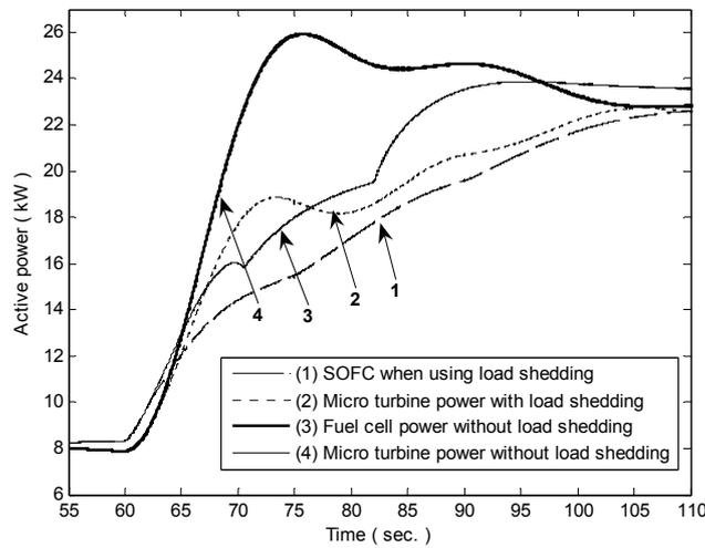
Fig. 15. Active power of micro turbine and fuel cell
