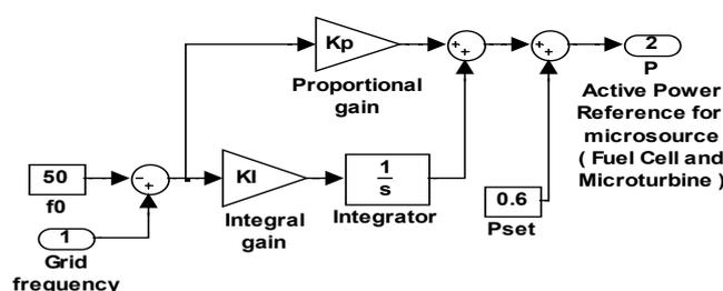
Fig. 4. Control of active power in controllable micro sources
