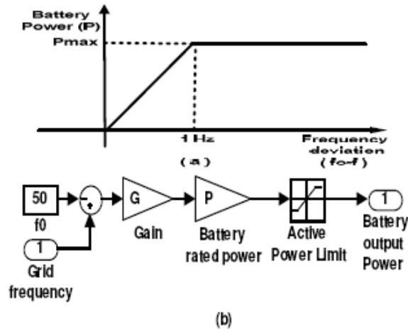
Fig. 7. Battery dynamic block diagram
