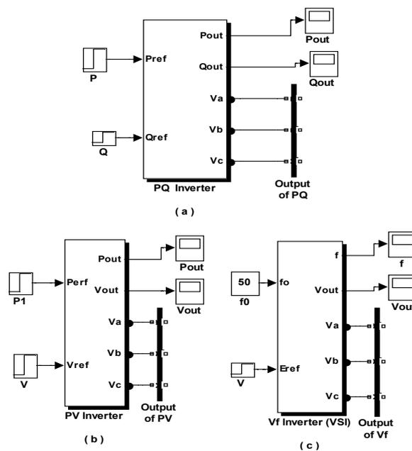
Fig. 2. Inverter control models
