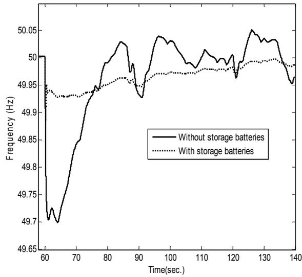
Fig. 8. MG frequency with and without storage batteries
