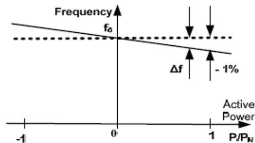
Fig. 6. Frequency droop control of Vf inverter
