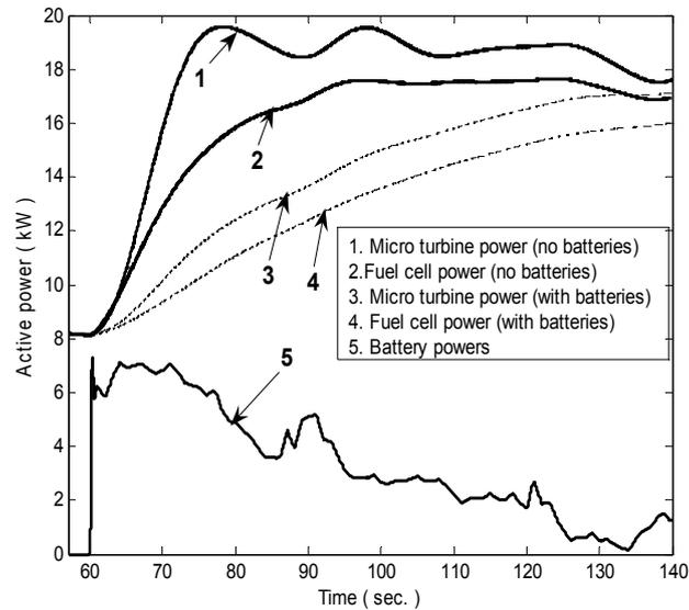
Fig. 11. Active power of SSMT, SOFC and batteries
