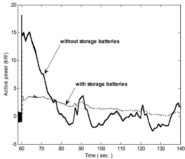
Fig. 10. Flywheel (Vf) injected active powers
