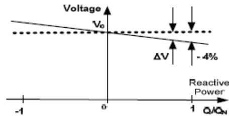
Fig. 5. Voltage droop control of the Vf inverter terminal
