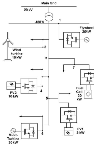
Fig. 1. Single line diagram of the studied MG
