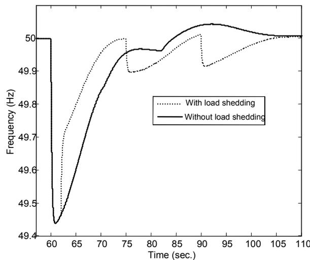
Fig. 12. MG frequency with and without load-shedding
