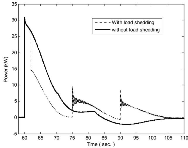
Fig. 14. Active power injected by flywheel
