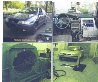
Fig. 4. The under study vehicle, embedded equipment, wind force and road friction physical simulator systems
