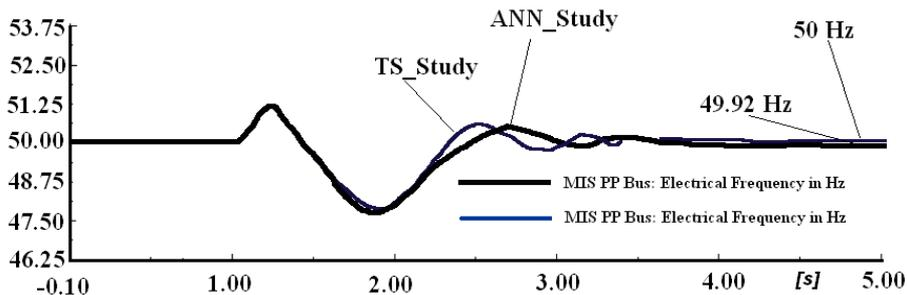
Fig. 10. Frequency response of M.S.C system in two different algorithms in case 3
