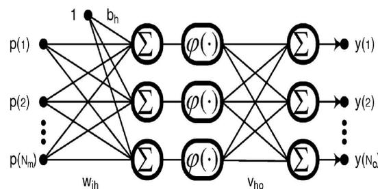
Fig. 1. Structure of a two-layered (or single-hidden-layer) feed-forward network
