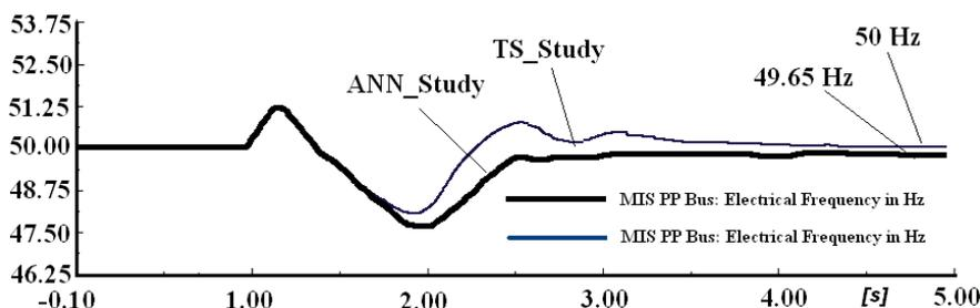
Fig. 12. Frequency response of M.S.C system in two different algorithms at different case5
