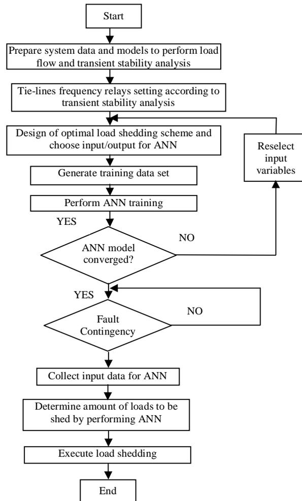
Fig. 2. Flowchart of ANN-based optimal load shedding
