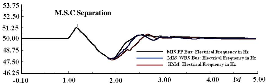
Fig. 9. Frequency response of M.S.C power system in case 2
