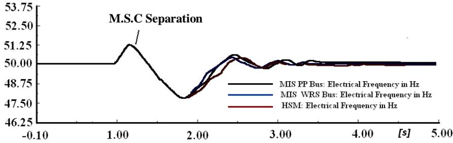
Fig. 8. Frequency response of M.S.C power system at case 1
