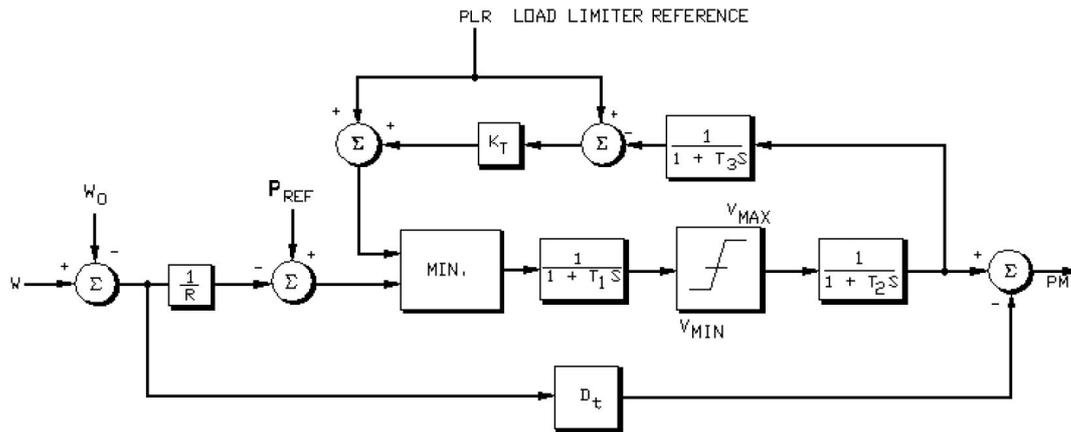
Fig. 5. Governor system for gas generator units in the M.S.C and E.R.E.C network
