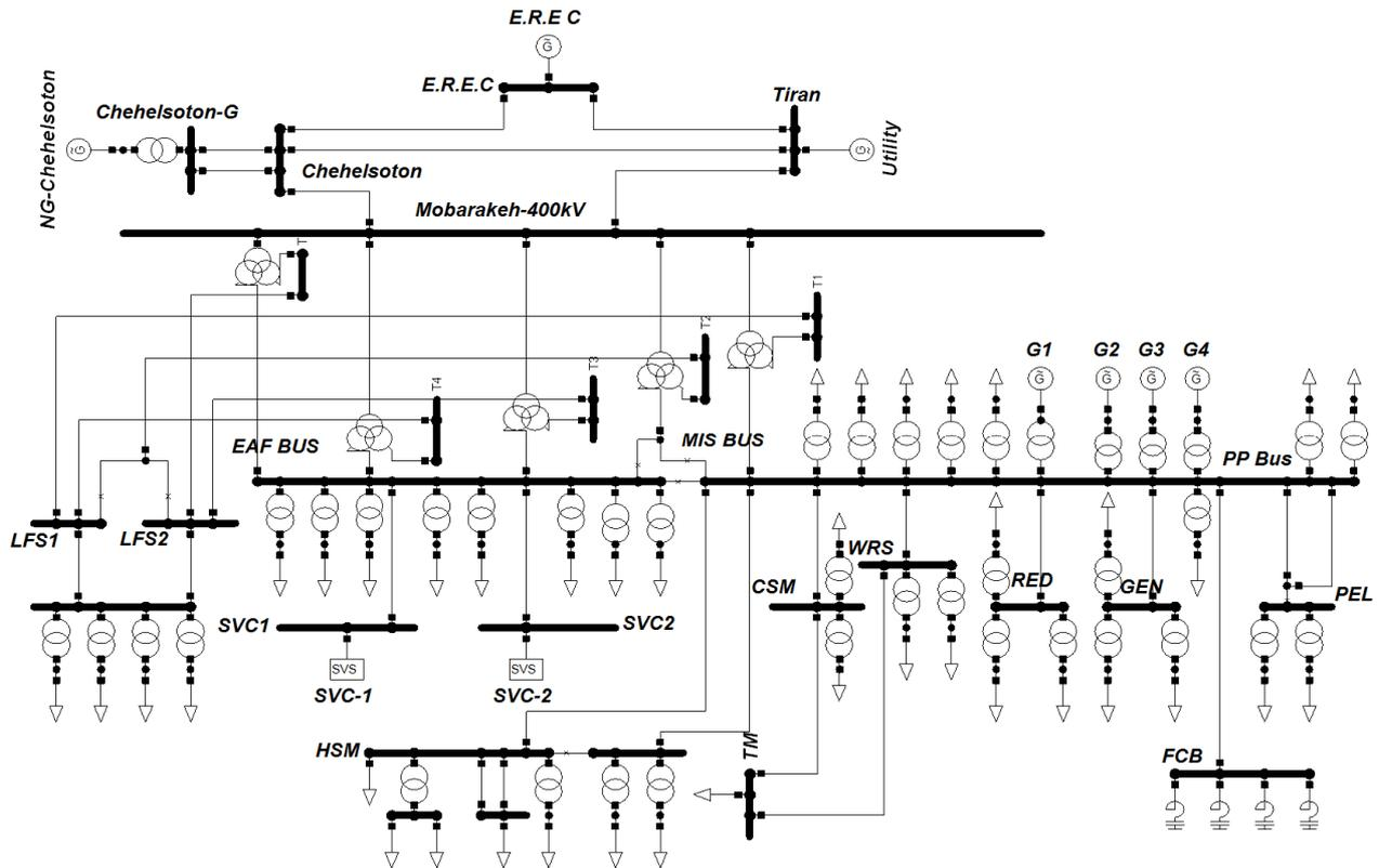
Fig. 3. M.S.C power system single line diagram
