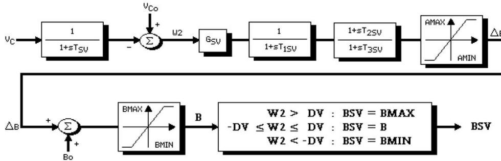
Fig. 6. SVC controller diagram in the M.S.C power system
