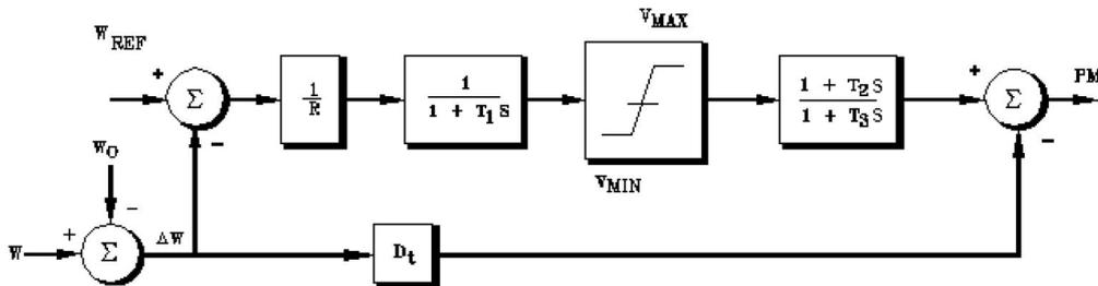
Fig. 4. Governor system for steam generator units in the M.S.C and E.R.E.C network
