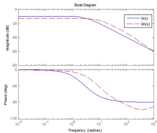
Fig. 4. Original system versus reduced system of order 2
