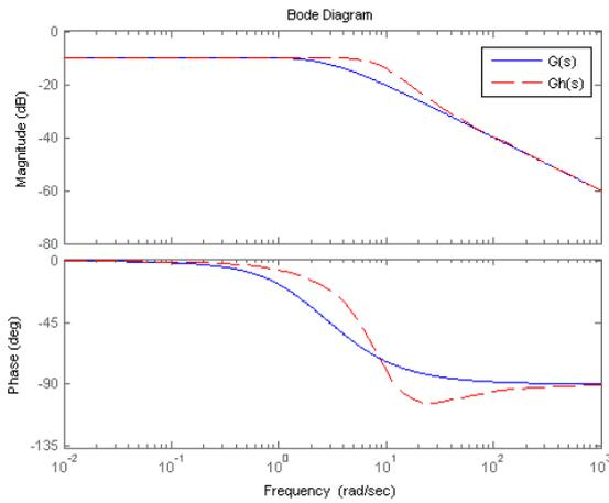
Fig. 3. Original system versus reduced system of order 3
