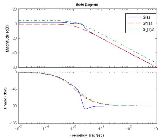
Fig. 6. Main system (blue solid line), Hankel reduced model (green dash-dot line), LMI based reduced model (red dash line)
