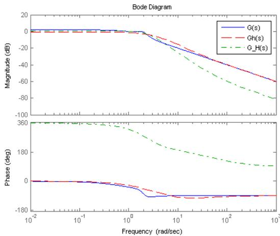
Fig. 5. Main system (blue solid line), Hankel reduced model (green dash-dot line), LMI based reduced model (red dash line)
