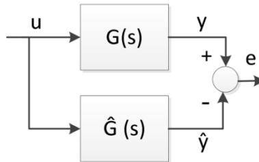
Fig. 1. Error system transfer function
