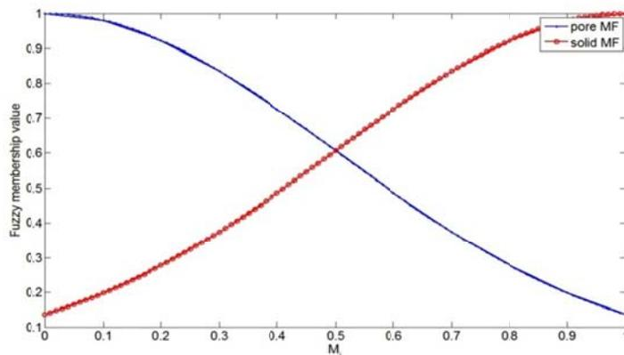
Fig. 2. The fuzzy membership function of being pore or solid pixel
